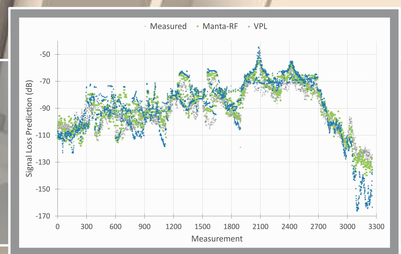
Comparison of signal loss predictions using Manta-RF and VPL [Liang & Bertoni 1997] against measured data from the Rosslyn, VA dataset (measurement locations shown at left).
